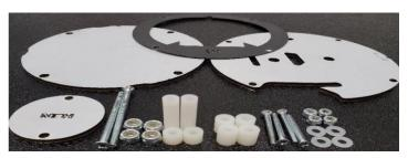
Rear mounting plate: Put (2) #6 x 2" Recessed Phillips head screws in rear mounting plate. Next, (2) #6 x  $\frac{1}{4}$ " Nylon spacers. Next, (2) #6 x 1" Nylon spacers. Next, (4) #6 Nylock nuts. Set 2 Nylock nuts aside you use them to mount Assembly to housing later. Tighten these down because these are going to be mounting points later.
