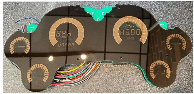
Place Acrylic over circuit board and overlay
