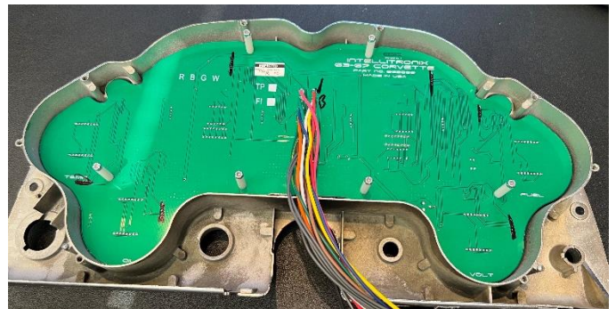
Insert circuit board assembly into housing
