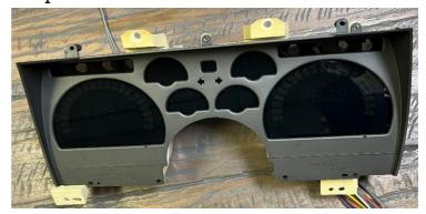
Place the new gauge assembly into the modified housing and attach the front bezel to the housing with the factory hardware. The new gauges will be wedged between the bezel and housing.
