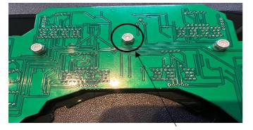
Secure the assembly using the lock nuts provided
