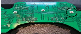
Lay nylon washers over the screw to protect circuit board
