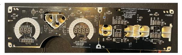
Line up the printed circuit boards into the factory plastic housing
