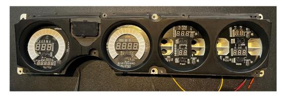
Line up the black factory cut out piece over the printed circuit boards
