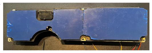
Line up the smoked acrylic lenses over the black factory cut out piece, you can use the provided double sided tape to hold the acrylic in place for easier install
