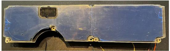
Secure the factory clear plastic lens over the assembly using the factory hardware and install into the factory bezel as normal.
