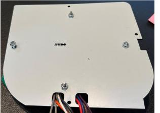
Secure the back plate to the assembly using the nylock nuts. You will reuse the factory mounting hardware to mount the tach board assembly into the bezel
