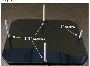
Insert the provided screws through the front of the smoked plexi glass *Be sure to remove the* protective film from both sides Step 3
