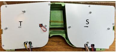
Insert the assemblies into the factory bezel and secure the backing plate to the bezel using the factory screws. You can now re insert the bezel into the dash cluster
