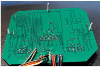
Place the circuit board over the screws and spacers
