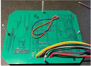
Place the circuit board over the screws and spacers
