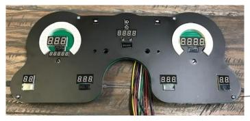
Attach overlay to the front of the circuit board using 4 #8-32 X 3/8" screws
